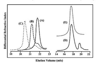
**Figure 2.** SEC chromatographs of: (A) PB homopolymer with approximate number average molecular weight  $(\overline{M}_n)$  10,000 g/mol, (B)  $(PB)_2$ -macroinitiator, (C) Living  $(PB)_2$ PI $^{(-)}$ Li $^{(+)}$  1st Generation Copolymer prior to linking with  $CH_3$ SiCl $_3$ , (D) Unfractionated 2<sup>nd</sup> Generation Dendritic Copolymer of the  $[(PB)_2PI]_3$  type and (E) Fractionated 2<sup>nd</sup> Generation Dendritic Copolymer of the  $[(PB)_2PI]_3$  type.
