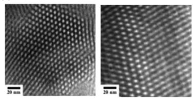
**Figure 3.** TEM micrographs of the  $[(PB)_2PI]_3$   $2^{nd}$  generation dendritic copolymers. Left image corresponds to the  $[(PB)_2PI]_3$ -10K sample and right image to the  $[(PB)_2PI]_3$ -20K sample. Both cases exhibit hexagonally close packed cylinders of PI (lighter domains) in the matrix of PB segments (dark domains).
